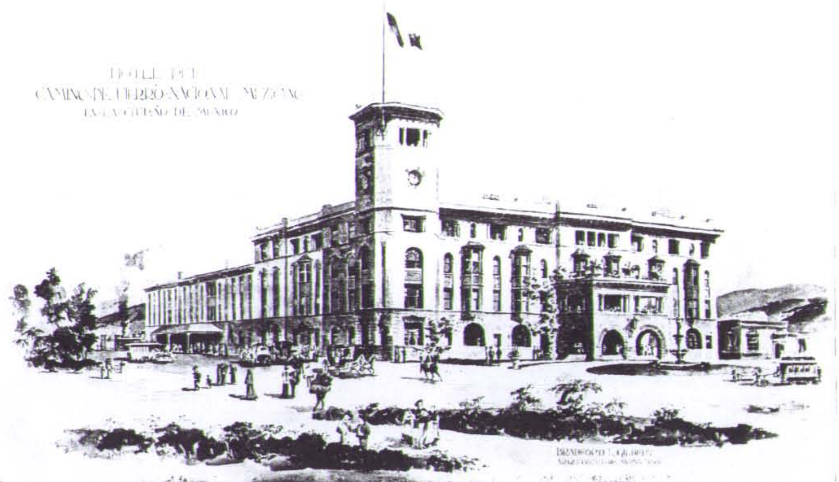
Proposed Construction of Tepetate and Stone. Dimensions Over All: 180 ft. x 200 ft., Four Stories in Height.
